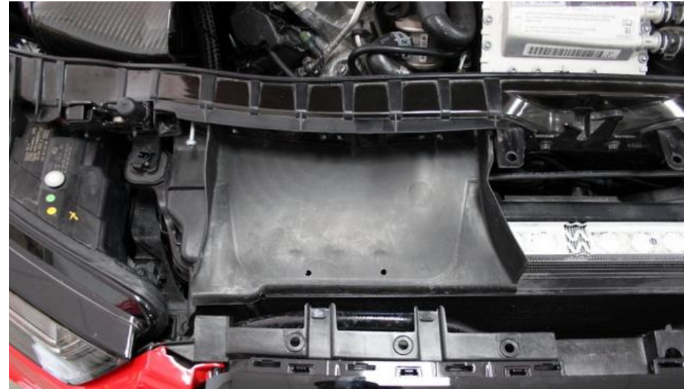
34. Attach the panel back into place. Make sure it is located properly and pushed back down onto the radiator.
