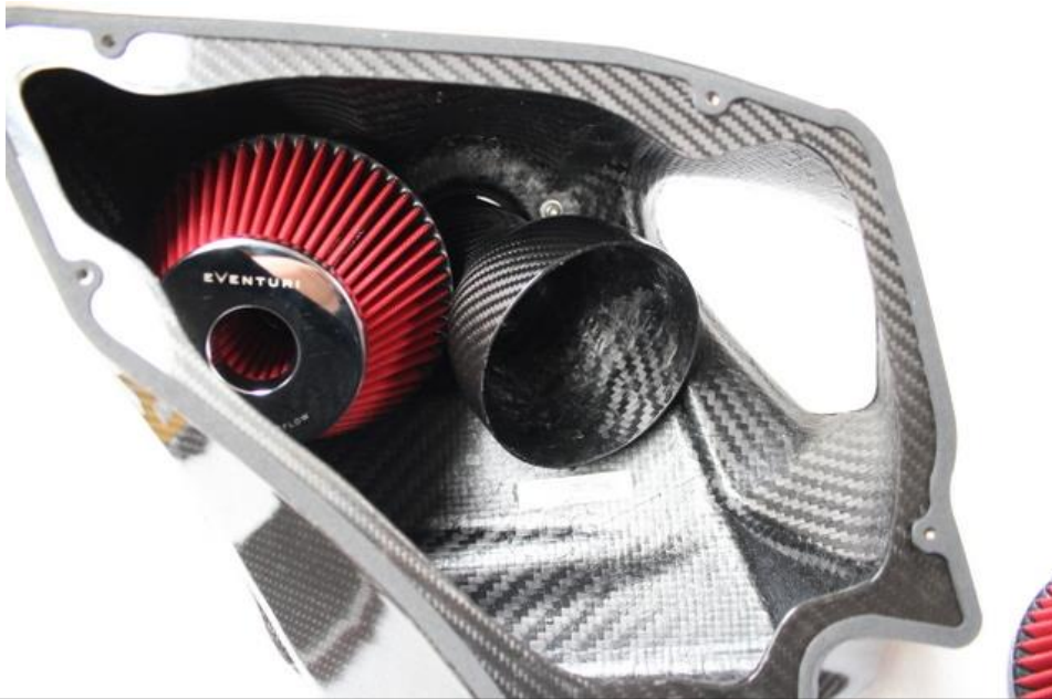
21. Push the tube all the way back to allow space for the second filter.
