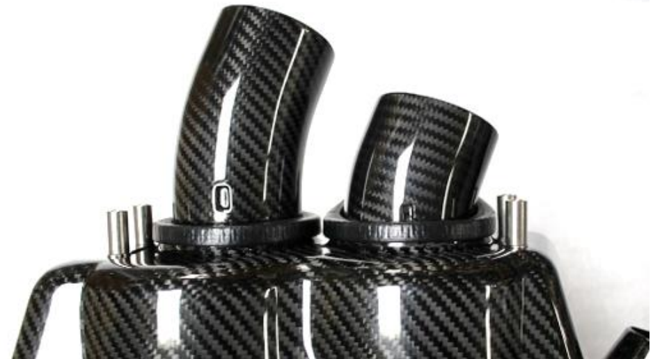
24. Push the tubes through and rotate so you can see the notches in the tubes as shown.
