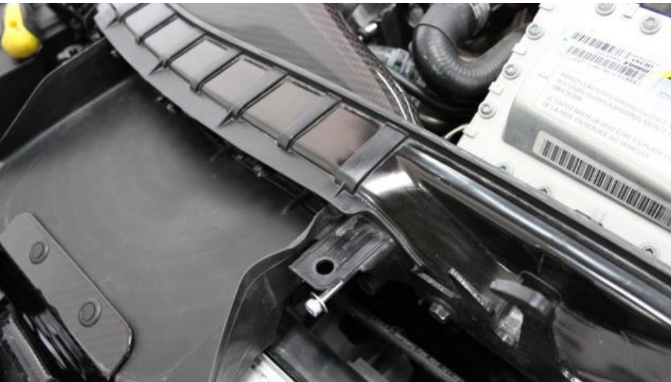
43. Push the bolt with washer through the panel and duct as shown.
