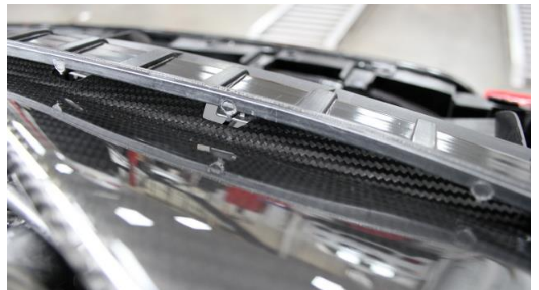
40. MAKE SURE the top of the carbon duct is above the plastic edge shown in step 37. This is important otherwise the duct will not be in the correct place.
