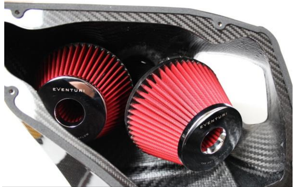
22. Push the filter onto the tube all the way and secure the clamp around the filter. It might be easier to pull the tube down for access to the clamp – see next step.
