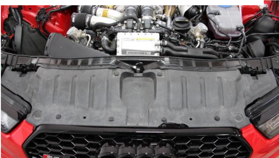
13. Remove the front slam cover by pulling out the plastic push rivets.
