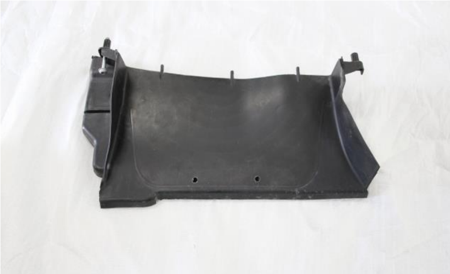
33. Drill 2 holes 6mm diameter.
