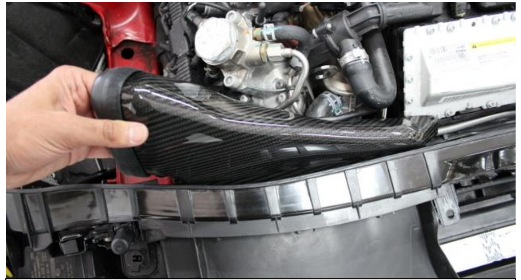
38. Rotate the duct as shown and place into location – then rotate to fit (next step). Ensure the top edge of the carbon goes above the edge shown in previous step.
