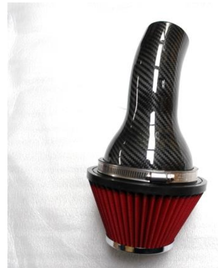
16. Assemble the filter to the SHORTER tube only. Push the filter as far as possible onto the carbon tube – make sure it is even all the way around and tighten the clamp.
