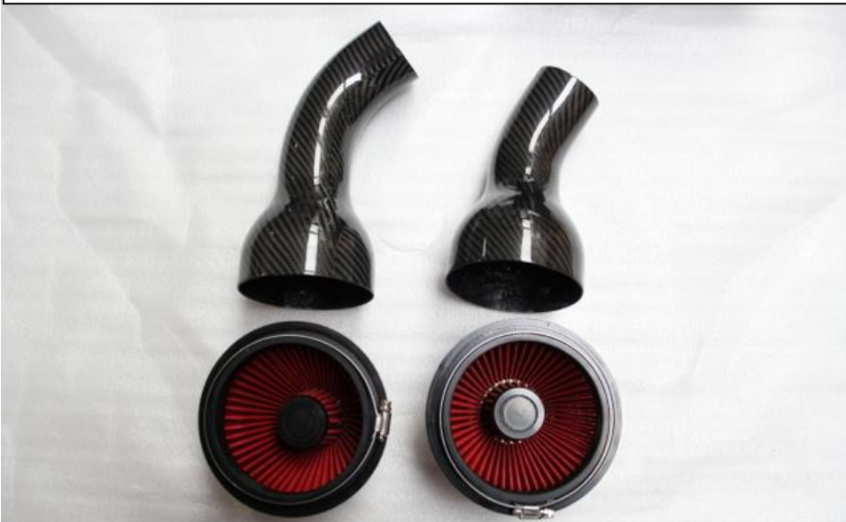
15. Now we will prepare the airbox. Start by taking the 2 inlet tubes and filters, you will notice one is shorter than the other.
