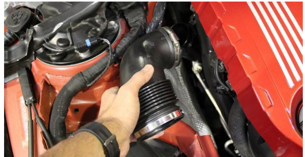
8. Loosen the remaining hose clamp on the intake tube and remove from engine bay.
