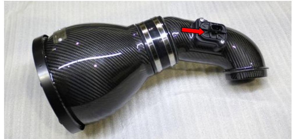
31. Assemble the LHS intake with the LHS tube (shorter tube) with the 80mm silicon coupler and 2 hose clamps. Orient the tube as shown here and in the next photo. When pushing the silicon coupler onto the intake – DO NOT PUSH ON THE FILTER ITSELF . Ensure airflow arrow on sensor is as shown.
