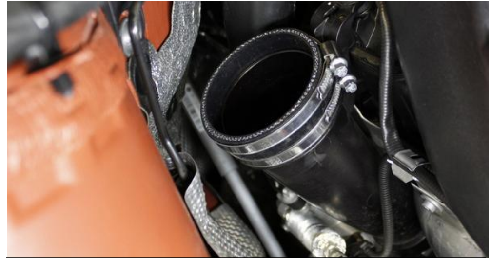
29. Taking the shorter 76mm coupler, push over the intake tube on the LEFT side of the engine. Make sure the coupler is pushed down fully and put two hose clamps around the coupler as shown. Tighten the LOWER clamp only.
