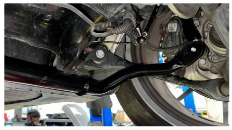
**Step 8**Grease the supplied bushings.
