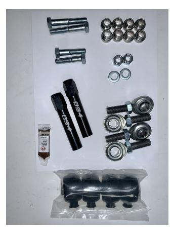
• Open anti-seize packets and apply to the end of heim joints, 1 packet should cover 2 joints.
