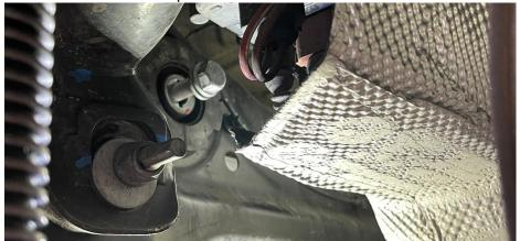
Torque the front hardware to 50Nm + 180°
