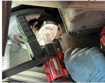
Using an 21mm socket, loosen the "front" subframe hardware. Leave about 5 threads engaged.
