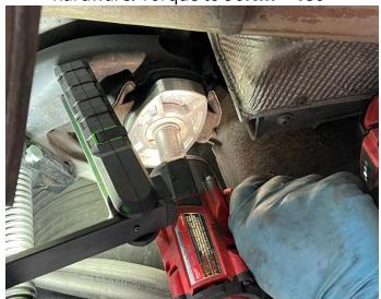
Using an 21mm socket, loosen the "front" subframe hardware. Torque to **130Nm + 180**°
