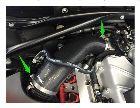
**Step 8** – Reinstall the small vent hose onto the supplied barb.
