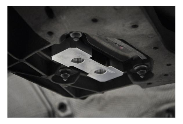
**Step 5** – Secure the 034Motorsport Transmission Mount Insert using the 10mm triple square bolts you removed in <u>Step</u> <u>2</u> and torque to 20 Nm. Blue Loctite is recommended. Yes, we provided an anchor link back to <u>Step 2</u> so that you wouldn't get lost. We're nice people like that over here.
