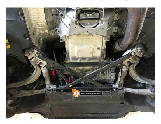
**Step 3** – Support the subframe brace with one hand to ensure that it doesn't fall on your head. Using the 18mm socket, 14mm triple square, and your superhuman strength, loosen the bolts that attach the stock subframe brace.
