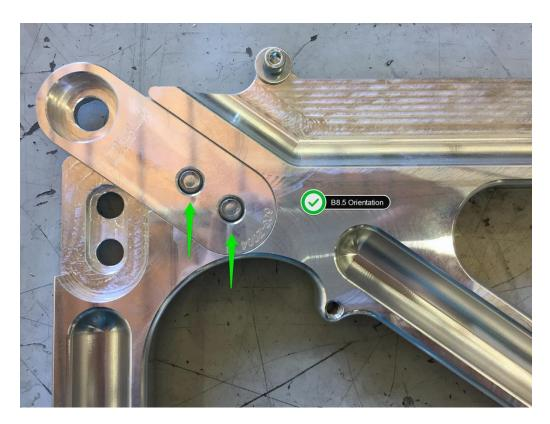
**Step 7** – Install the 034Motorsport X-Brace using new bolts. **(Pre-Facelift)** Torque the six M12 hex head bolts to 90 Nm + 135 Degrees. **(Facelift)** Torque the four M12 hex head bolts to 90 Nm + 135 Degrees. Torque the two M12 triple-square bolts to 90 Nm + 90 Degrees. Marvel at your work!
