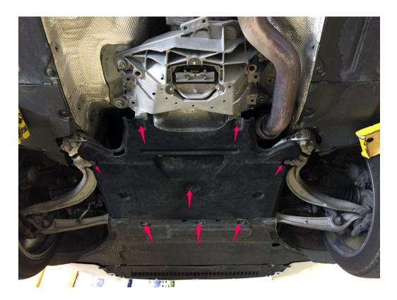
**Step 2 – (Facelift)** Remove the two plastic factory clips securing the power steering cooler lines to the stock subframe brace. **(Pre-Facelift)** Use a 10mm socket to remove the nut securing the power steering cooler to the subframe brace.
