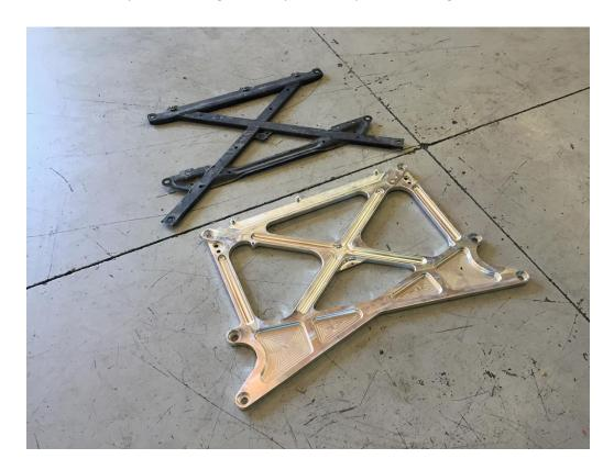
**Step 6** – In this step, install the Modular X-Brace Inserts in the proper orientation for your vehicle. Torque the provided M10 screws to 55 Nm using a 6mm allen driver. (Facelift) The inserts should install diagonally, as pictured below. (Pre-Facelift) The inserts should be installed straight up and down.
