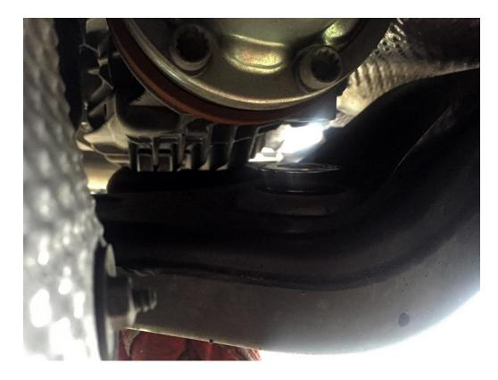
**Step 4** – Install the bottom insert (505-2018) into the void in the bottom of the differential mount bushing, as pictured below. Make sure that the features on the insert line up with the voids in the differential mount. Secure using the 16mm hex head bolt you removed in Step 1, and torque to 55 Nm.
