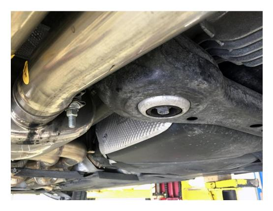
**Step 2** – Raise the front of the differential approximately 3 centimeters to gain access to the top of the front differential mount bushing. Ensure that you have enough space to slip the top insert (505-2017) into the top of the front differential mount bushing.
