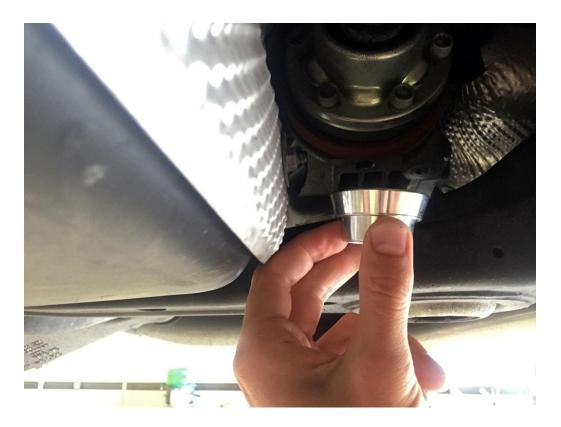
**Step 3** – While the differential mount is raised, slip the top insert (505-2017) into the void in the top of the differential mount bushing. Ensure that the top insert (505-2017) is properly seated in the differential mount bushing, and slowly lower the front of the differential back down.
