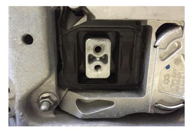
**Step 4** – Press the shiny new 034Motorsport Transmission Mount Insert into the void. The orientation of the 034Motorsport logo is not important. Or is it? It's not, but it might matter to you.
