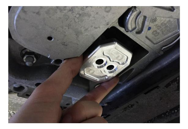
**Step 5** – Secure the 034Motorsport Transmission Mount Insert using the 10mm triple square bolts you removed in <u>Step</u> <u>2</u> and torque to 20 Nm. Blue Loctite is recommended. Yes, we provided an anchor link back to <u>Step 2</u> so that you wouldn't get lost. We're nice people like that over here.
