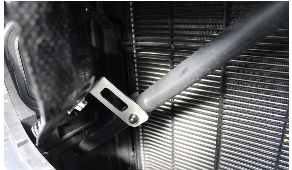
18. Push the clip onto the strut brace.
