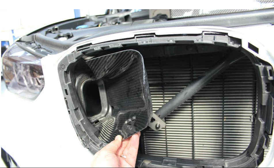
17. Place the LHS Scoops into the left opening – the clip on the bracket should go onto the strut brace – see next step.
