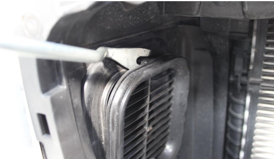
15. The grills are held in place with a tab on top and at the bottom. Carefully prise the clips out and remove the grills.
