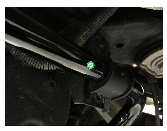
**Step 7** – Install the Billet Aluminum Sway Bar Mounting Brackets with the supplied washers and bolts, ensuring that the grease fittings are in the correct orientation. Snug up the hardware, but do not tighten fully.
